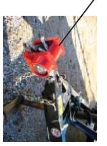
securing the chains and hitch. Big Red LOCK is on a trailer tongue
